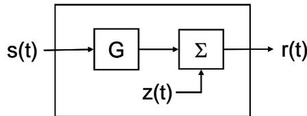
If the input is  $s(t) = \tilde{s}(\omega_0)e^{i\omega_0 t}$  and there is an additive noise  $z(t)$  with power spectrum  $P_z(\omega)$ , then the quantity  $\frac{1}{T} F(r, \omega_0, T, 0) \equiv \frac{1}{T} \int_0^T r(t)e^{-i\omega_0 t} dt$ , when calculated for data lengths  $T$  that are a multiple of the period  $2\pi / \omega_0$ , has a mean value  $\tilde{s}(\omega_0)\tilde{g}(\omega_0)$  and a variance  $\frac{1}{T} P_z(\omega_0)$ .
