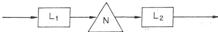
Fig. 3. A linear/nonlinear/linear "sandwich" model. This is a model which may apply to the nonlinear pathway of the Y retinal ganglion cells. L_1 is a linear filter, the prefilter, N is a nonlinear element. In the retina N seems to be a rectifier or threshold element. L_2 is a linear filter, the post-filter.
