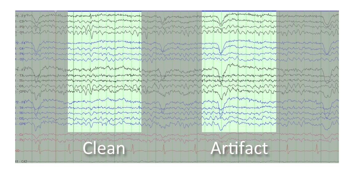
**FIGURE 1** A typical run of EEG with both clean and noisy segments. A typical clean segment is highlighted on the left; artifact (in this case an eye blink) is highlighted on the right.
